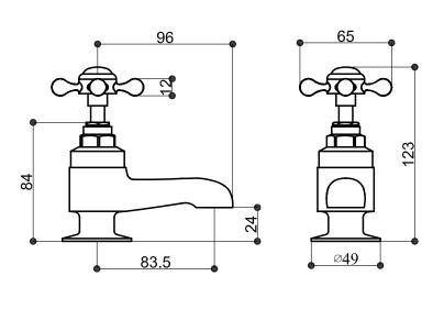
Identify the hot tap and position into the bath on the left hand, from the underside of the bath fit the rubber washer and then the nut. Making sure the tap is in the right position tighten the nut to secure the tap to the bath.
