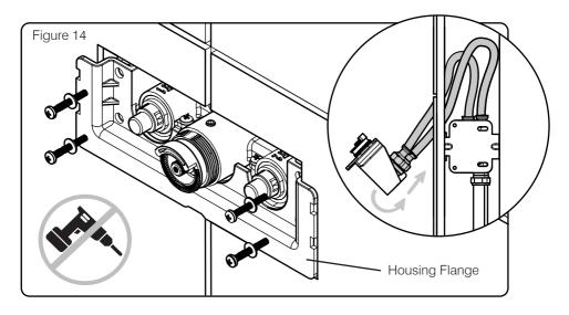
13. Lift the valve and push the hoses back through the access hole, making sure the hoses do not kink (Figure 14). Position the valve flat against the tiles and line up the fixing holes with those on the metal installation frame. Secure the valve to the fixing frame.
