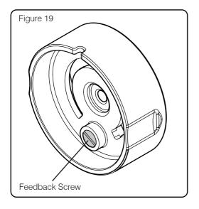
18. Once installed, the handle should click as it rotates. This click can be adjusted to give more feedback when in use.
