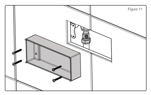
10. Remove the tiling guide, allowing access to the pipework behind the tiled wall. Keep these screws safe as they will be used to mount the valve. From this position the isolation valves should be visible and accessible through the access hole.
