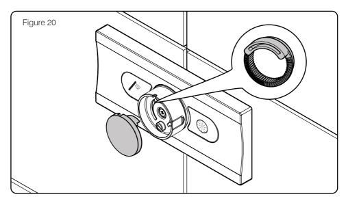
19. With the handle installed, the centre dial can be pushed into place. The dial has a tab that fits into the temperature stop ring via a gap in the handle. To remove the dial for maintenance, line up the notch in the centre dial with the notch on the handle and use a small screwdriver to separate the two parts.
