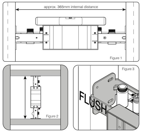
2. Position the installation frame between the two stud timbers at a suitable height for its final installation position. The front of the frame and the front of the timber stud should be flush (Figure 3). Use a spirit level placed on the tiling guide to make sure the installation frame is level both front to back and left to right. Once level remove the tile guide and keep the fixing screws safe for later steps.
