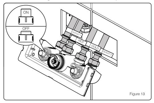
12. Working from left to right, using the labels as a guide, connect the hoses to the valve. Ensure the hose from the hot supply is connected to the inlet marked hot on the valve. Do the same for the cold supply. Ensuring all outlet buttons are in the 'OFF' position (Figure 13), turn the water supply back on at the isolation valve. Do not overtighten the hoses as this may damage the rubber washers.
