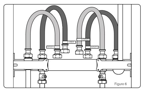
5. Connect the flexible hoses to the manifolds - ensure that each hose has a rubber washer inserted at each end to create a watertight seal. Once connected, label each hose with the corresponding inlet / outlet - this will help easily identify which hose is which during later installation stages.
