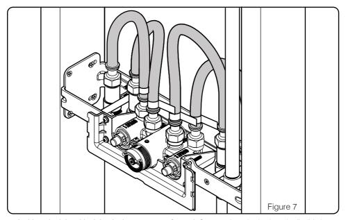
6. At this point it is critical that leak tests are performed. Connect the valve body to the flexible hoses - the hot and cold inlets are marked with red and blue paint on the valve. Turn on the water supply and test the system for leaks. Push the buttons for each outlet and check all connections are fully sealed.
