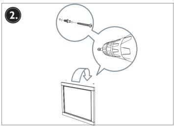
Drill two holes in the marked positions using an 8mm drill bit to a depth of 55mm. Insert the wall plug supplied in the ficing screw, leaving sufficient head showing to slide into the mirror wall brackets.
