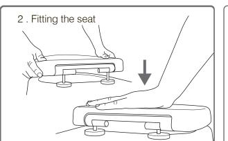
Align and insert the hinge anchors into the hinges on the seat and firmly press down until the seat is engaged into position. Adjust the hinge anchors to make sure the seat lines up with the edges of the toilet pan. When you are satisfied the seat is in the correct position, remove the seat from the hinge anchors (see step 3) and fully tighten the screw (shown in step 1). Place the cover plates over the hinge anchors. Replace the seat and 'push' into position.
