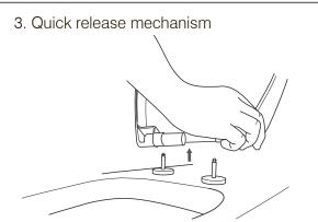
This toilet seat is designed for quick and easy removal when cleaning the toilet pan. To quickly release the seat, lift the lid and seat up to a vertical position. From there, lift one side of the seat up to disengage the pin followed by the opposite side. the seat should easily lift away from the pins. To replace the seat align the sockets with the pins and firmly press down until the seat is engaged into position.
