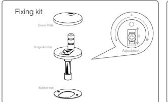
Maximum adjustment of the pin position is achieved by rotating the hinge anchor around the screw (adjustment A in the parts diagram above). Further fine adjustment of the pin position can be achieved by sliding the screw in the adjustment plate (adjustment B).
