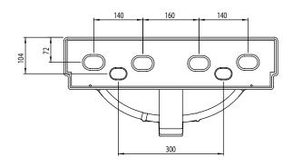
Diagrams not to scale All dimensions in mm tolerance of +/-5mm
