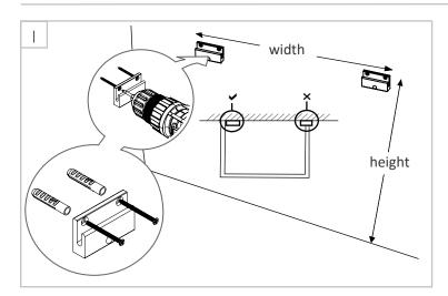
Mark the location of each of the wall mounting plates ensuring that they are positioned inside the sidewalls of the unit. Use a spirit level when marking to ensure that the mounting plates will be level. For each mounting plate drill two holes in the marked positions using a 8mm drill bit to a depth of 55mm.
