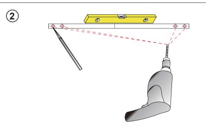
Use the template supplied to determine the final installation position, mark the fixing hole positions in pencil.
