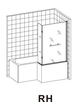
L Shape Bath Screen is ok to be installed in left hand or right hand. Please choose the direction you want and follow below steps. Below steps are based on left hand. For right hand, please turn the screen panels upside down and follow below steps in mirror direction.
