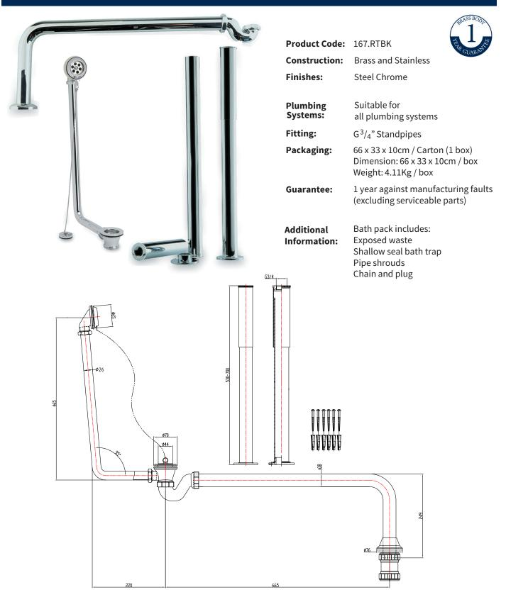
All dimensions are in milimetres unless otherwise stated. The information contained on this page was correct at date of issue. Fitting dimensions are provided as a guide only. Some variation may occur due to manufacturing tolerances. We pursue a policy of continuing improvement in design and performance of our products and so reserve the right to change specifications without prior notice.
